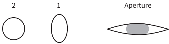
Fig. 7c. When wire 1 is deformed into a vertical oval, the aperture opens, especially in the axial portion (shaded).
