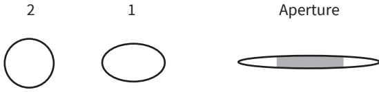
Fig. 7b. When wire 1 is deformed into a horizontal oval, the aperture closes, especially in the axial portion (shaded).
