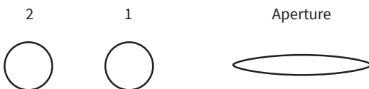
Fig. 7a. Schematic representation of the effects of wire deformation on the reed's aperture. In this "neutral" adjustment, wire 2 is round, wire 1 is round, and the aperture is a medium ellipse.
