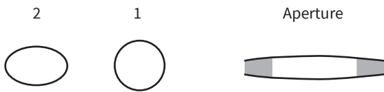
Fig. 7d. When wire 2 is deformed into a horizontal oval, the aperture opens, especially in the off-axial portions (shaded).
